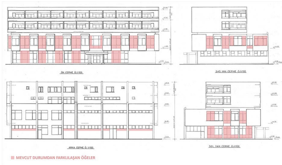
Figure 8. Representation of the modifications on the elevations of the 1984 dated project (TÜLOMSAŞ Archive, 2019).
